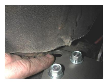
2. Mark the hole in the bottom of the frame and drill with 5/16" bit. Use the 3/8" self-tapping bolts supplied and bolt the bracket to the frame. Mark and drill the remaining holes.
