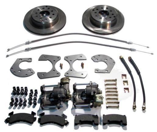
This kit is for Ford 9" rear axles with the large Torino (3.15") style bearing. This kit is designed to work with axles with either GM 5 x 4.75 Bolt Pattern and 7/16" wheel studs or Ford 5 x 4.5 Bolt Pattern and 1/2" wheel studs. Rotor center measures 2.78".
