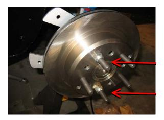
Take out the caliper and notice how Bracket #2 and the contour of this caliper shown below fit.
