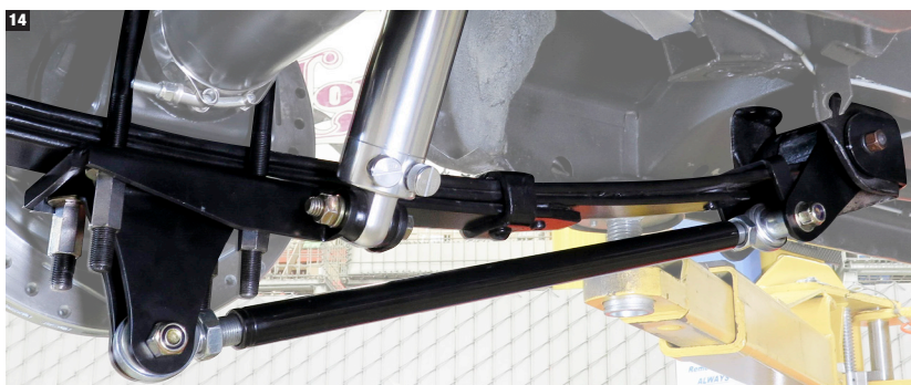
14. With the car sitting at ride height, adjust the length of the traction bars by loosening the locking nuts and twisting the bar. Adjust the traction bars so the anti-torque strap is just touching the leaf spring. With the vehicle sitting at ride height, tighten all hardware to the proper specifications.
