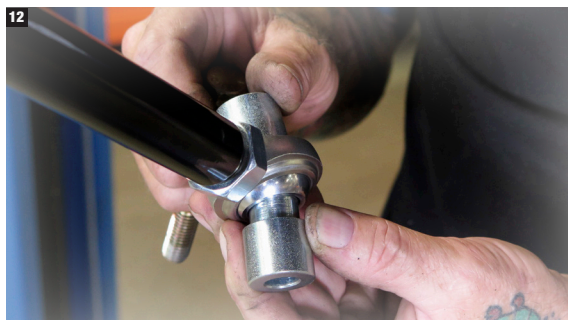
12. Fit the front of the traction bar with the provided spacers.
