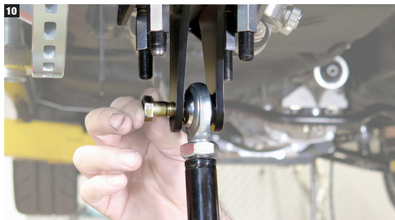
10. Attach the traction bar to the rear mounts but wait until the end to fully tighten.
