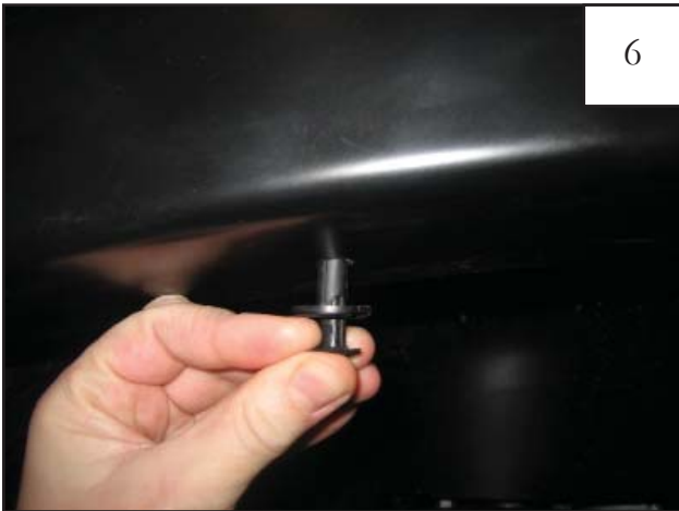
Install two supplied Retainers (RV1-P006).
