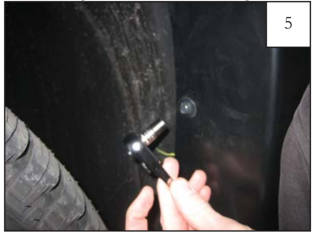
Holding flare in position on fender, reinstall factory screws removed in Step 4. If necessary, use awl (or similar pointed tool) to locate holes.
