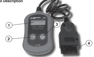
**1. LCD DISPLAY**--Indicates test results. It is a backlit 2-line display with 8 characters on each line.
