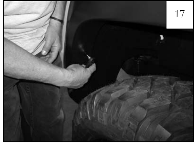
Place flare on vehicle lining up holes in flares with factory screw holes.
