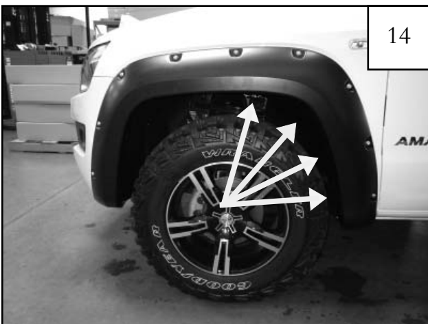
Using T-25 Torx bit, reinstall factory screws in 4 remaining Flare holes. Fully tighten all screws starting with the newly installed Screws (SW1-0058) in two forward hole locations while pressing in on flare to ensure it is snug against sheet metal.
