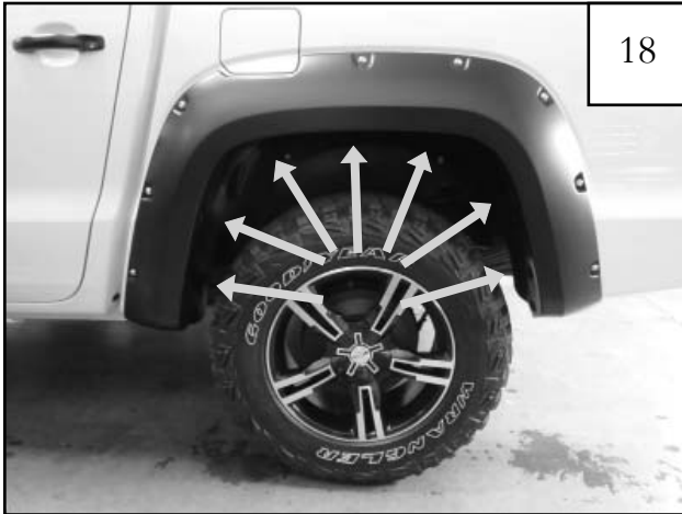
Using T-25 Torx bit, install 7 factory screws. Fully tighten all screws while pressing in on flare to ensure it is snug against sheet metal.
