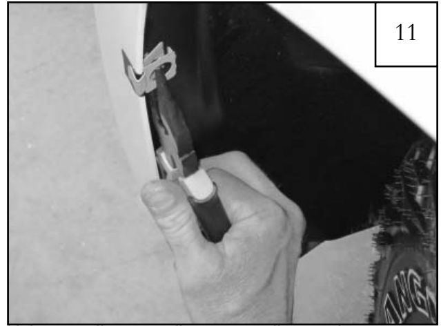
Using needle nose pliers, snap clip together to secure to the vehicle.
