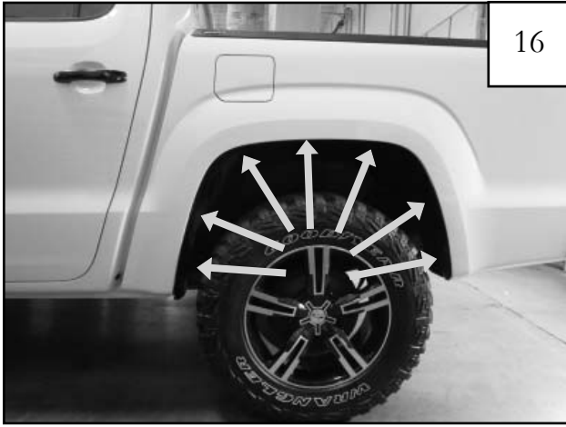
Using an T-45 Torx bit, remove 7 factory screws. Retain screws for reinstallation.
