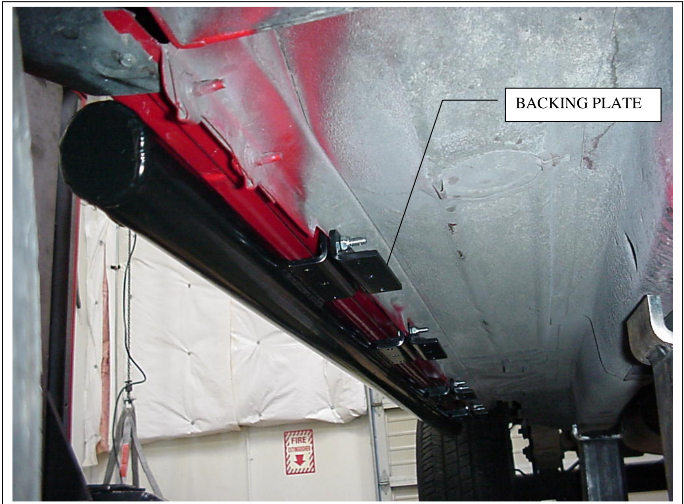
Figure 7, Rock Slider installed with backing plates.
