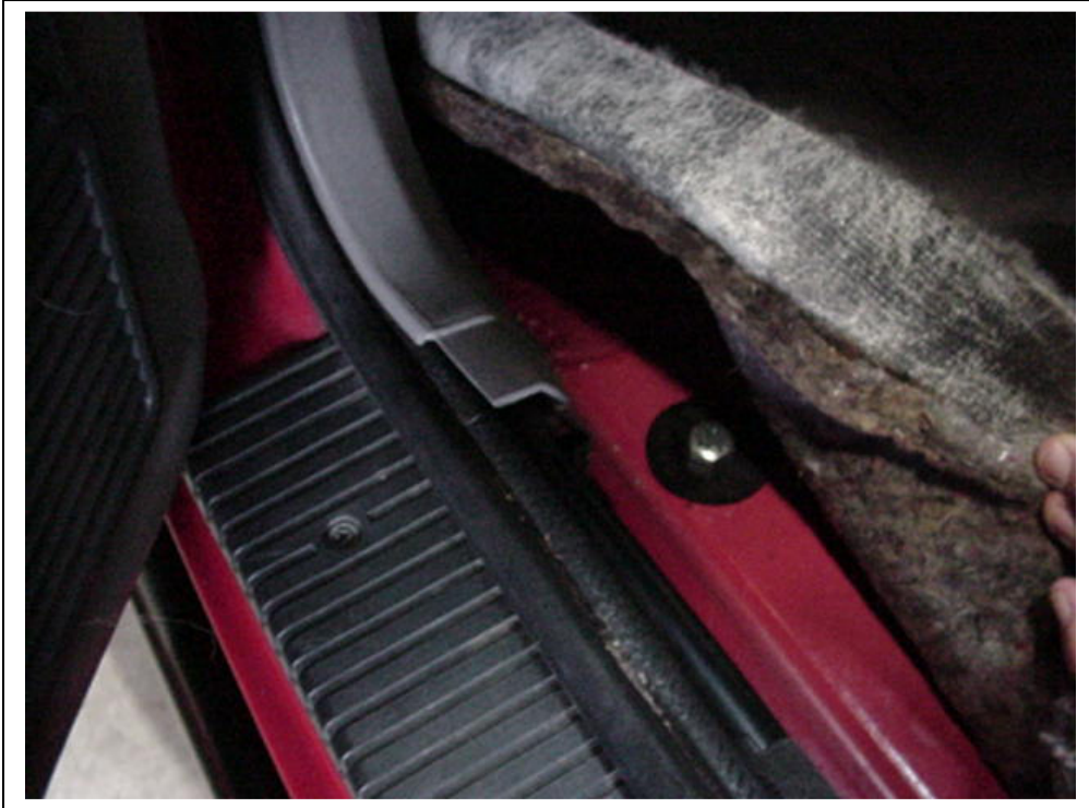
Figure 10 , Front floor hole under carpet.
