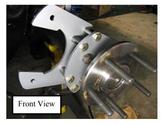
Slide the rotor onto the studs. The rotors are drilled for both Ford and Chevy bolt pattern. Hand thread two lug nuts to seat the rotor in place for test fitting.
