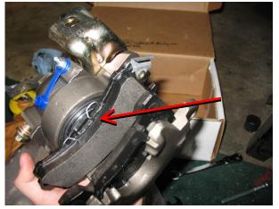
Slide the caliper into position, have the brake pads go on each side of the rotor and the two mounting holes on the caliper will match up with the two holes in Bracket #2.
