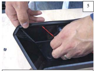
Press edge trim into place along the top edge of the flare in one foot increments, pulling red vinyl backing free as you go.
