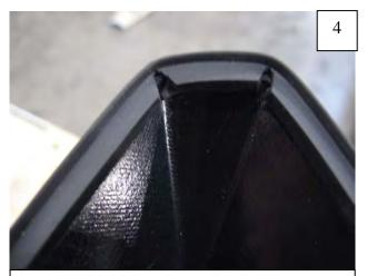
At sharp corners, use a utility knife to notch a "V" in edge trim, taking care not to cut front face of edge trim (four places each part)
