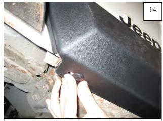
Attach underside edge of the Rocker Panel to the vehicle using supplied Tuf-Lok® fasteners, pressing Tuf-Loks through slots and into factory holes.
