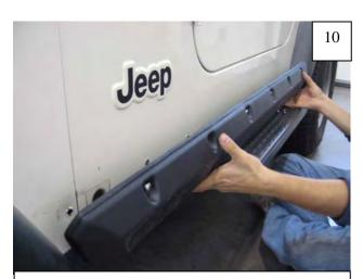
Gently position part on vehicle, centering between fender flares (about 1/4" to 3/8" space on each side). Take care not to press the part onto vehicle until properly positioned.
