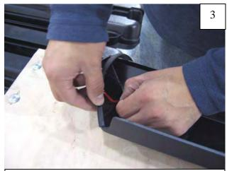
Applying the adhesive side of the edge trim to the inner side of part, affix edge trim to the top edge of the part (the portion that comes in contact with vehicle).
