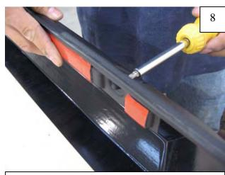
Using supplied Torx bit, start a screw/washer through each pocket into the indent in the inner piece (4-5 turns). Do NOT tighten!
