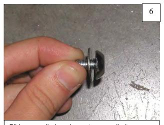
Slide a supplied washer onto a supplied screw.
