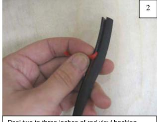
Peel two to three inches of red vinyl backing away from edge trim tape.
