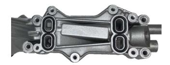
STEP 7: Install original oil cooler onto new oil filter housing.
