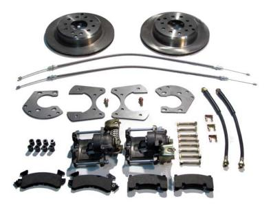
This kit is for either Mopar 8  $\frac{3}{4}$ " or Mopar 9  $\frac{3}{4}$ " (Dana). This kit is designed to work with axles with either GM 5 x 4.75 Bolt Pattern and 7/16" wheel studs or Mopar / Ford 5 x 4.5 Bolt Pattern and  $\frac{1}{2}$ " wheel studs. Rotor center measures 2.78".
