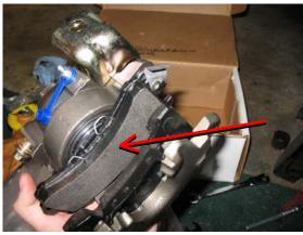
Slide the caliper into position, have the brake pads go on each side of the rotor and the two mounting holes on the caliper will match up with the two holes in Bracket #2.
