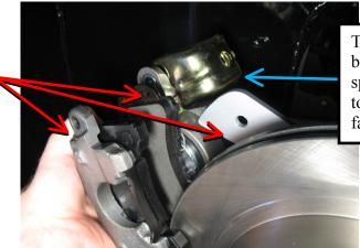
The zinc plated bracket with spring attached to it needs to face upwards. With the caliper on the rotor and in Bracket #2 you can use the two caliper bolts to secure the caliper in place using a 3/8" allen wrench and torque to factory specs.
