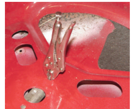
Photo #10: With the pull cable and spring attached to the clutching drum, install clutching drum to the trunk latch. Clip a pair of vise grips on the latch shaft to hold the drum in place while connecting the trunk lock cylinder.
