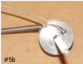
Photo #5a & 5b & 5c: A 1/8" stranded cable connects to the drum of the clutching device. The cable wraps around the drum and when pulled by the electric solenoid, the drum will rotate and unlock the trunk without the lock cylinder turning.
