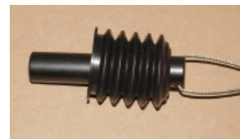
Photo #10: With the pull cable and spring attached to the clutching drum, install clutching drum to the trunk latch. Clip a pair of vise grips on the latch shaft to hold the drum in place while connecting the trunk lock cylinder.
