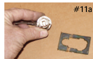
Photo #11a & 11b: The trunk lock cylinder is held in place with a retaining clip P/N 54-39 . Feed the lock cylinder through the trunk lid and connect it to the clutching device. Next, anchor the lock cylinder in place using the retaining clip. Now, remove the vise grip pliers from the shaft on the inside of the trunk. Turn the key making sure there is no binding or dragging of the clutching device between the lock cylinder and trunk latch.
