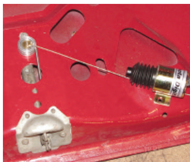
Photo #7: The electric solenoid mounts on the driver's side of the trunk lid between the inner and outer skin. When the solenoid is activated, it will pull the stranded cable and unlock the trunk latch. With the modified trunk latch installed in the trunk lid, install the clutching device into the latch on the inside of the trunk lid. Now, place the electric solenoid at about 4:00 o'clock to the clutching device aiming the ram of the solenoid in the direction of the pull cable and drill two 1/4" mounting holes.
