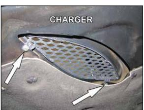
25. On vehicles equipped with hood vents: If the vehicle is to be driven during inclement weather it is recommended the shield be installed onto the hood vent to guard, the air filter from concentrated water. Remove the two bolts that secure the factory vent grid.
