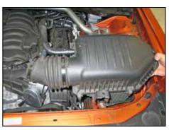
7. Lift up and remove the complete intake track from the vehicle.
