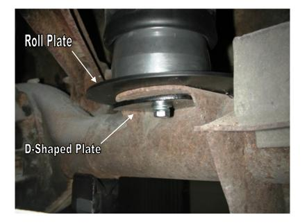
7. Place the 7.25" air spring roll plate over the cut down coil spring retainer. Pull the lower piston down to the plate.
