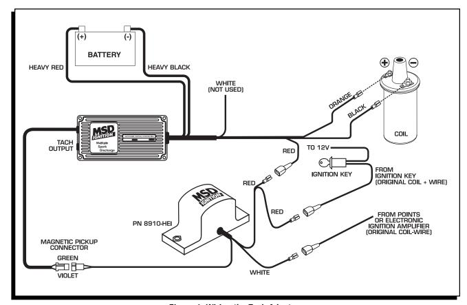
Figure 1 Wiring the Tach Adapter.
