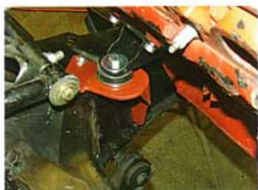
Photo #10: The big block engine complete front mounting kit uses a GM transmission crossmember. This crossmember works great for automatic or standard transmissions and with dual or single exhaust. In January 2001 we introduced a new tubular transmission crossmember P/N 19-153 to replace the stock GM type crossmember.
