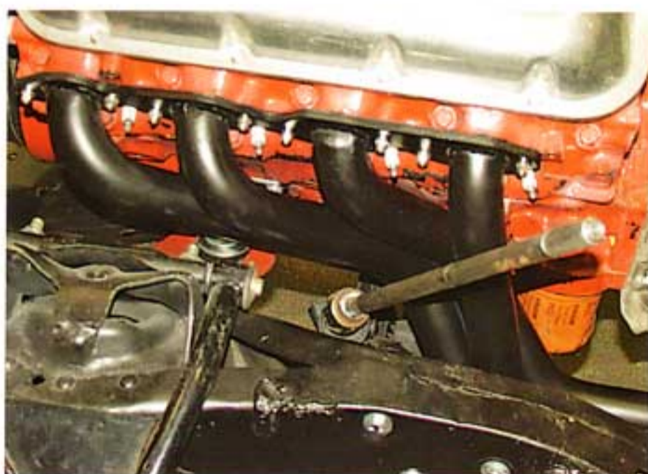
Photo #15: The 2" tube headers are designed to be used with rack and pinion steering only due to lack of clearance around the large primary tubes. The tubes are pulled up close to the engine block to properly clear the steering shaft for the rack and pinion.
