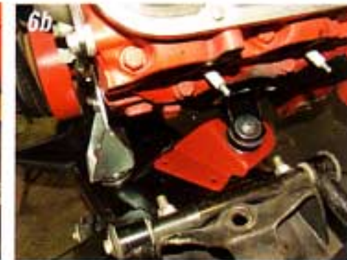
Photo #6a & 6b: With the frame brackets bolted to the engine brackets, the lower legs of the frame brackets will be on the back side of the front engine crossmember. The top of the frame brackets will be to the outside of the factory front engine mounting holes.
