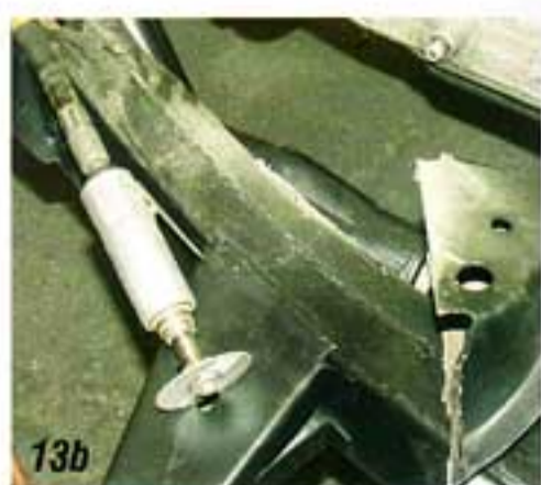
Photo #13a & 13b: With the engine now side mounted and the transmission installed, the factory frame horns can be removed. These can be cut from the frame with a torch or cut-off wheel.
