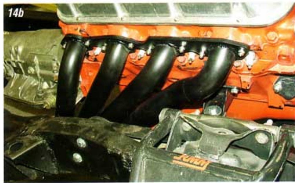
Photo #14a & 14b: Now for the icing on the cake: big tube 2" headers for a big block engine! A new 2" big tube header set P/N 24-56 and 24-56C has been developed for higher performance engines that require larger tube headers. These headers have an extra thick 5/16" flange at the cylinder head for leak-proof sealing and a huge 3" collector and 2" primary tubes. These headers will flow more than enough for any big block in a Tri-Five car. They will also work with any of our Turbo or Flowmaster exhaust systems.
