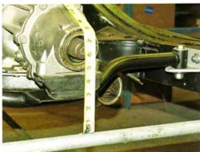
Photo #12: When installing the transmission crossmember, position it so that the center output shaft of the transmission measures 6-1/2" up from the bottom of the frame.
