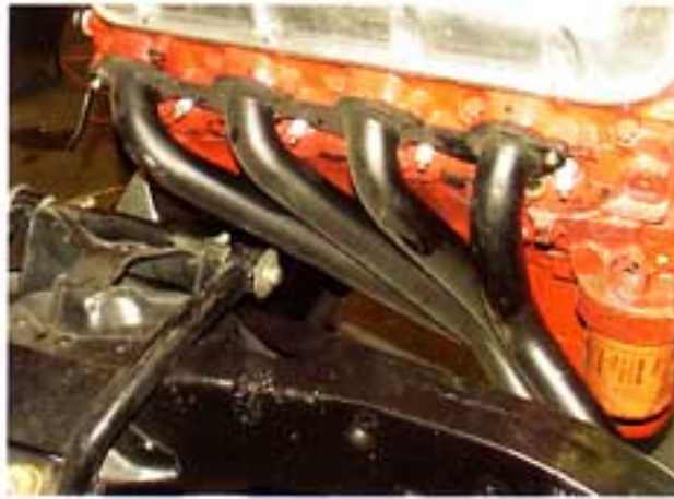
Photo #2: The 1-3/4" headers that are designed for the front mount kit exit just under the rear engine mounting brackets. The 3" header collector hangs about 1-1/2" below the bottom of the frame.
