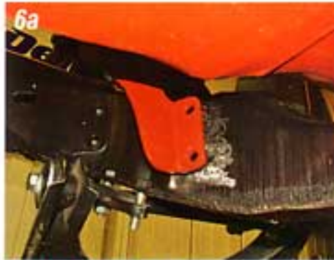
Photo #6a & 6b: With the frame brackets bolted to the engine brackets, the lower legs of the frame brackets will be on the back side of the front engine crossmember. The top of the frame brackets will be to the outside of the factory front engine mounting holes.
