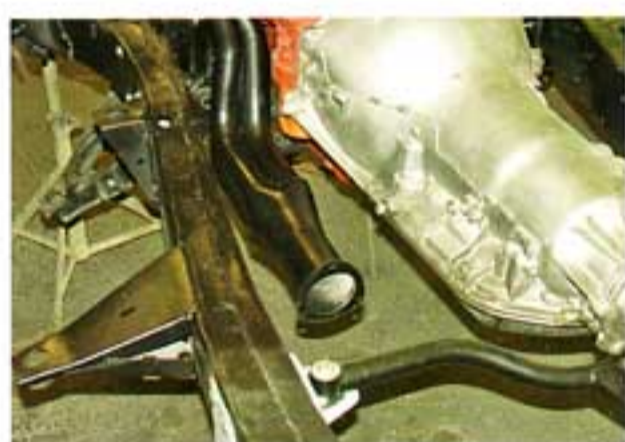
The tubular crossmember has a more custom look and takes up less space than the GM crossmember.
