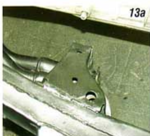
Photo #13a & 13b: With the engine now side mounted and the transmission installed, the factory frame horns can be removed. These can be cut from the frame with a torch or cut-off wheel.
