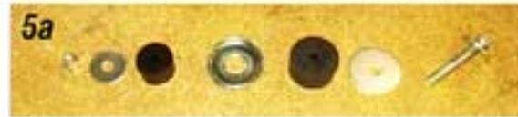
Photo #5a & 5b & Diagram: The side mounts bolt to the frame brackets with a 7/16" X 3" grade 5 bolt with washers, rubber grommets and a locking nut. Support the engine with an engine hoist or a jack under the oil pan and bolt the frame brackets to the side mount brackets.
