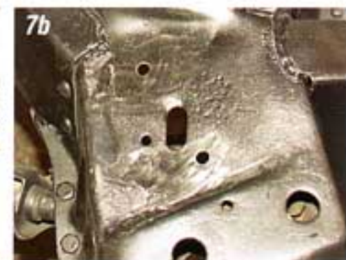
Photo #7a, 7b & 7c: Mark the engine crossmember where the eight 3/8" holes will need to be drilled. Now raise the engine up out of the way and drill the eight mounting holes.
