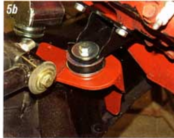
Photo #5a & 5b & Diagram: The side mounts bolt to the frame brackets with a 7/16" X 3" grade 5 bolt with washers, rubber grommets and a locking nut. Support the engine with an engine hoist or a jack under the oil pan and bolt the frame brackets to the side mount brackets.
