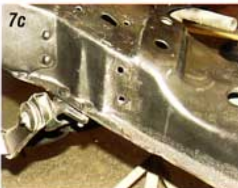
Photo #7a, 7b & 7c: Mark the engine crossmember where the eight 3/8" holes will need to be drilled. Now raise the engine up out of the way and drill the eight mounting holes.
