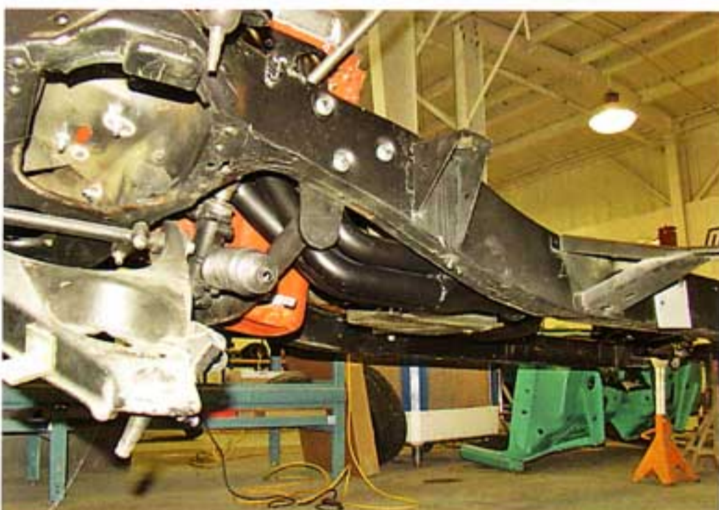
Photo #16: The P/N 24-56 and 24-56C headers are designed to tuck up inside the frame for plenty of ground clearance, which is great for lowered cars. These headers will work with automatic or standard shift transmissions.
