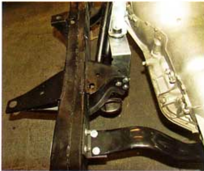
Photo #2: The 1-3/4" headers that are designed for the front mount kit exit just under the rear engine mounting brackets. The 3" header collector hangs about 1-1/2" below the bottom of the frame.
