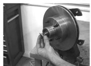
Step 5: Next install the outer wheel bearing and spindle washer.
