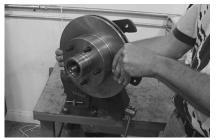
Step 4: With the inner wheel bearing and seal installed, place the disc brake rotor onto the spindle.
