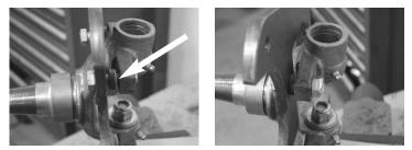
Step 2: The disc brake bracket mounts to the rear of the spindle. Two 1/4" spacers are installed at the top of the spindle between the disc brake bracket and spindle. Two 7/16" X 2" grade-8 bolts and nuts hold the disc brake bracket to the spindle. The lower rear ear of the disc brake bracket fits on the inner side of the spindle.
