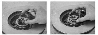
Step 3: Pack the wheel bearings with a high quality disc brake grease. Install the inner bearing and seal in the back side of the disc brake rotor.
