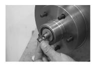
Step 6: A spacer is installed between the spindle nut and spindle washer.
