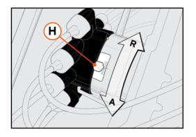
C) For advanced tuning, the Stromberg e-FIRE distributor also allows adjustment of the total mechanical advance and advance curve. Please visit the Stromberg Tech Center at www. stromberg-97.com for further advice.
