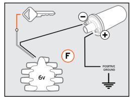
black wire to the negative ( - ) side of the ignition coil. Connect the red wire to the positive ( + ) side of the ignition coil or other power source controlled by the ignition switch. (see D)
