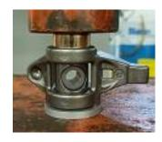
Press the washer/bushing down and as the washer gets close to going over the trunnion shaft, check to make sure it's still centered, then press the bushing down until it's flush with the rocker body. Install both snap rings and repeat the process to the other rocker arms.
