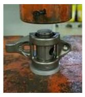
Put a light coat of oil or assembly lube inside the other bushing and place on top of the rocker, sliding it over the trunnion and centering it on the rocker arm housing bore.
