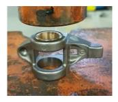
Place one of the 2 installation washers (thinner with smaller hole than the removal washer) under the press, then set the rocker arm on top with the side the bushing is in down and trunnion sticking through the center of the washer.
