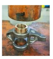
Press the bushing into the rocker arm body just until it is flush with the outside. Lift up the rocker arm and place a light coat of oil or assembly lube on one end of the new trunnion and insert it into the rocker body and installed bushing.
