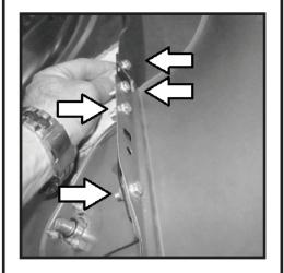
6 - Installation of fender is the reversal of steps (1)-(21) of the snorkel instructions. Reinstall windshield bracket. If windshield bracket does not line up correctly. floating nut plates in a-pillar can be boken free with a screwdriver to allow for additional movement.
