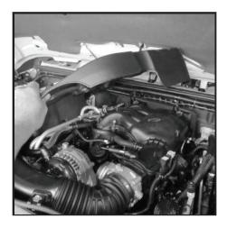
43 - (NOTE: 3.6L application only) Using a 10mm socket remove the two retainer bolts holding the (3.6L) air hose to the radiator. Do not discard bolts. They will be reused.
