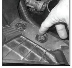
68 - Insert (2) M8 x 35 bolts with (2) M8 flat washers through lower air box mounting holes and rubber grommets. Apply a small amount of sealant to washers.
