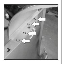
25- With spot welds cleared carefully remove upper cowl from fender. NOTE: Fender can be damaged if welds have not been opened completely.
