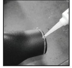
80 - Snorkel main body should rest in place as shown. Snorkel body should be fitted tight to inner frame. Some vehicles may require the pinch seam (arrow) to be rolled for proper fitment. Check antenna cable position.
