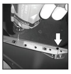
32 - Carefully trim extra metal from inner antenna support bracket as shown. DO NOT cut too deep or damage to outer fender may result. A Dremmel tool with a cut off wheel is recommended.
