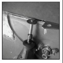
fender along marked lines. Cut should start in the middle of outer cut line (arrow). Cut should be 1/8" away from rolled edge. Cut in each direction towards 7/32" terminating holes (arrows).
