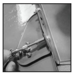
3 - Align bracket to the holes of upper fender cowl plate and fender. Plate will be placed under fender as shown.
