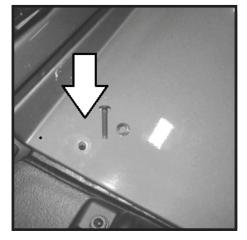
87 - Slide nut plate under 86 - Locate cowl nut plate. Nut plate is used to snorkel body as shown. secure cowl cover and Working from engine snorkel body to "Z" compartment align mounting holes. Start one M6 Phillips head screw to hold in place.
