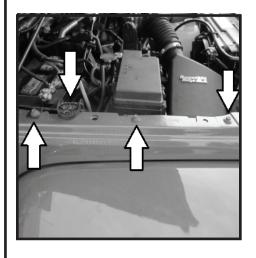
109 - Tuck drain tube up behind inner fender liner and between lower fender and inner pinch weld. as shown.
