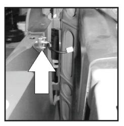
18 - Top cowl section of fender may be adhered to body. A small flat head screw driver or putty knife can be used to release cowl section from body. painters tape can be used to protect windshield paint if leverage is needed to release top cowl section.
