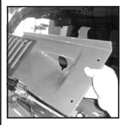
85 - With cowl cover removed tighten "Z"- bracket. Reinstall cowl cover and reinstall drivers side M6 x 20 screws and washers. Reattach center retainer clips removed in step (5).
