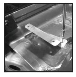
79 - Add a bead of sealant to the upper section of air tube (arrow). Slip main snorkel body and coupling over air tube as shown. Slide 3" clamp over 45 deg elbow but Do Not tighten.
