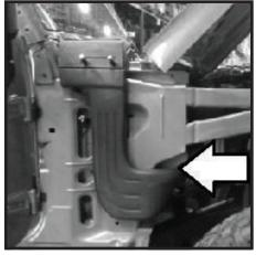
78 - Slide 45 deg elbow onto main body lower outlet. Secure 3" clamp around elbow Do Not tighten. Smooth and clean extra sealant from snorkel body.
