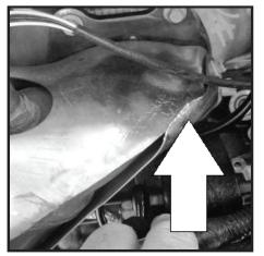
51 - With adjustments made insert tube and place mounting tab behind brake line mounting bracket. Secure 10mm bolt but do not tighten at this time. Final adjustment of air tube will be done later.
