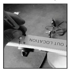
31 - Allow steel to cool before touching. Remove cut section from fender. Care should be taken when handling rough cut steel. 29- With guide holes marked and guide holes drawn drill 1/8" centering holes into fender. Use a 7/32" drill bit to enlarge 1/8" guide holes. NOTICE: A wood block should be placed under marked hole as described in steps 23&24. Wood block will protect the fender if drill bit grabs panel.
