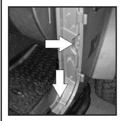
105 - Reinstall all remaining bolts removed in steps (8) through (13). Secure all bolts but do not tighten at this time.
