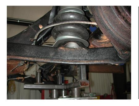
10. Bolt the lower mount to the bottom of the air spring using a 3/8" x 3/4" bolt, lock washer and flat washer. Before tightening, make sure it aligns with the lower arm.
