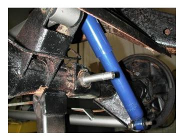
2. Attach the bottom of the shock to factory shock stud using the ½" Nylok nut & flat washer supplied.
