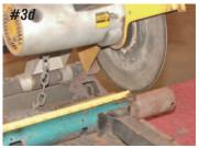
**Photo #3a & 3b & 3c & 3d:** The mast jacket and shift tube both need to be shortened to the same length. Using a chop saw or band saw, cut the bottom of the mast and shift tube off to exactly 27-1/4" overall length.
