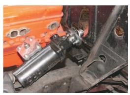
Photo #1: With the power steering box and coupler installed there is only about 1" of clearance between the coupler and firewall.
