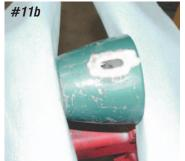
**Photo #11a & 11b:** Since this car has a floor shifter, the shift collar is fully inoperable. If you wish, you may remove the old shift handle boss from the collar and with a little body work it can be made to look like a shift lever was never there. Good luck!
