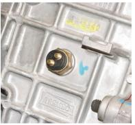
*Photo 17:* There are several electrical senders on the Tremec transmission case. The upper forward 2-pin sender on the driver's side of the transmission is the sender for the back-up lights. To connect the back-up lights to the sender, connect one of the pins of the sender to a key on fused
