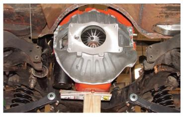
**Photo 9:** You may install the Tremec using the stock cast iron bellhousing if you desire. The aluminum bellhousing P/N 08-23 is a reproduction of the mid to late 60's GM bellhousing and can be used with side engine mounts only. The bellhousing bolts to the back of the engine with six supplied  $3/8" \times 1-1/4"$  bolts and lock washers.
