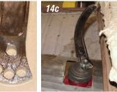
*Photos 14a, 14b & 14c:* A straight shifter arm **P/N 08-403** or a curved arm **P/N 08-402** is available for the **P/N 08-401** shifter. The curved arm works best with the bench seat. The arm has three lower adjusting holes,
