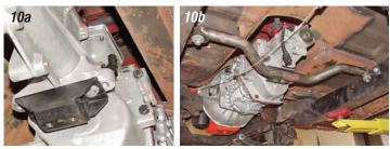
**Photos 10a & 10b:** The Tremec transmission is bolted to the bellhousing with the four supplied 1/2" X 1-1/2" bolts and lock washers. The tailshaft mount **P/N 19-26** is bolted to the transmission case with two supplied 10 millimeter metric bolts and lock washers. The transmission mount bolts to the supplied transmission crossmember **P/N 19-153** with two 7/16" X 1" bolts, flat washers and lock washers.
