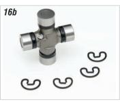
*Photos 16a & 16b:* The Tremec transmission uses a Ford C-6 automatic driveshaft slip yoke P/N 19-299. P/N 19-300 U-joint will adapt the Ford style yoke to the Chevy driveshaft.
