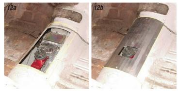
*Photos 12a & 12b:* The Tremec transmission case is fairly large and will make contact with the stock transmission hump. Tunnel **P/N 31-350** is a 16 gauge panel that can be installed in place of the stock hump to provide enough clearance for the Tremec case. The panel can be welded in or held in with tech screws. The stock carpet will still work perfectly.
