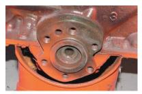
*Photo 6:* A new brass pilot bushing is included with the clutch and pressure plate kit. The bushing is installed in the rear crank hub to support the input shaft of the transmission on the flywheel side of the clutch
