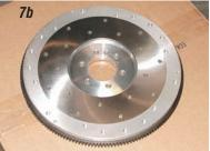
*Photos 7a, 7b, 7c & 7d:* The flywheel **P/N 08-409** is for an internally balanced small block or big block engine and will accept a 10-1/2" or 11" clutch and pressure plate. The flywheel is held to the crankshaft with six 7/16" standard transmission flywheel bolts **P/N 19-61** and serrated lock washers. Always use a small amount of thread locker on the flywheel and pressure plate bolts. Torque the flywheel bolts to 65 ft./lbs.
