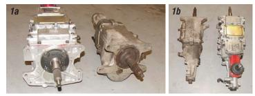
*Photos 1a & 1b:* The Tremec 5-speed transmission P/N 08-400 has the same bellhousing bolt pattern as the early model GM Muncie and Saginaw 3 and 4-speed transmissions.
