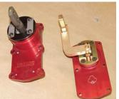
**Photo 4:** If the stock front bench seat is going to be used and adjusted forward, or if you prefer the shifter to be in a position similar to the 3 or 4-speed transmission, the McLeod offset shifter **P/N 08-401** will need to be used. This shifter offsets the shifter arm 2" to the left (driver's
