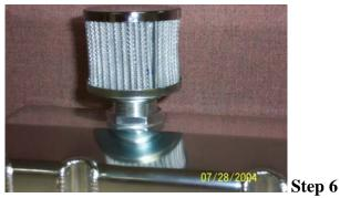
Install the washer, and then the nut. Be sure not to over tighten the nut. You can now put whatever breather you want into the baffle, as long as it fits a 1 1/4" grommet.
