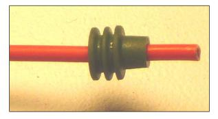
Slide the wire seal over the un-stripped wire as shown in the photo to the left. Doing this over an un-stripped wire will prevent the copper strands of exposed wire from penetrating the inside of the seal making it difficult to slide the seal onto the wire insulation.
