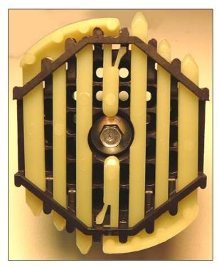
The white "combs" found in the kit are used as a terminal position assurance. These are extra security to ensure the terminals stay in their pin location. These "combs" are installed into the connector only after the wires being used are installed into the connector. Remember, any unused cavities will require a plug to be installed.
