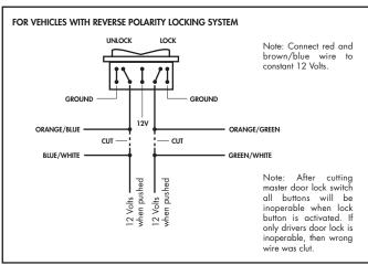
This system has a switch instead of an actuator in the drivers door. You will need to mount an actuator (GT series) in the drivers door to control your locks. Wiring diagram comes with actuator (GT series)
