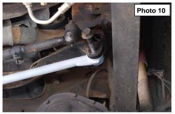
17. Using a 18mm socket and wrench, install the front shock absorbers in the factory location, part # 650328 hydraulic/ 650380 gas charged shock using hardware included in kit. Tighten the upper shock nut and lower bolt to 75 ft/lbs.
