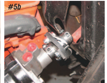
Photo #5a & 5b: The coupler is held to the steering box shaft and steering column shaft with set screws and lock nuts.
