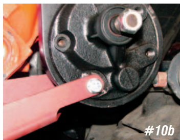
Photo #10a & 10b: Place the pump into the power steering pump bracket. The rear stud is secured to the bracket with a supplied flat washer, lock washer and nut. The front of the pump is held to the bracket with a supplied 3/4" long bolt and lock washer.
