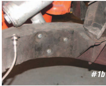
Photo #1a & 1b: The original steering box is bolted to the frame with three 3/8" carriage bolts and nuts. The stock mast jacket (steering column) protrudes through the firewall about 3-1/2". The steering shaft that connects the steering box to the steering wheel is part of the steering box and not removable.
