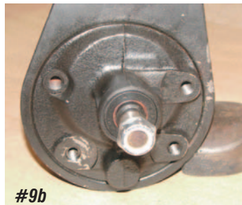
Photo #9a & 9b: There are two studs on the back of the power steering pump P/N 53-28 . The lower stud keys into the rear slot on the power steering pump bracket. On the front of the pump there are four 3/8" holes. The lower hole is used to attach the pump to the power steering pump bracket.
