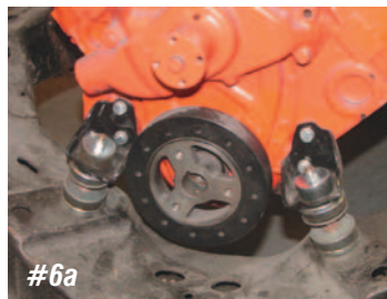
Photo #6a & 6b & 6c: The original front motor mounts attach to the front of the engine on each side of the harmonic balancer. The driver's side mount will be replaced with a combination left front motor mount and power steering pump mounting bracket. This bracket can also be used as the power steering pump bracket only if the engine is side mounted. Using an engine hoist or floor jack under the oil pan, slightly raise the engine to take the load off the front engine mounts.
