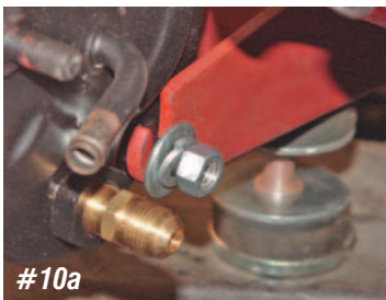
Photo #10a & 10b: Place the pump into the power steering pump bracket. The rear stud is secured to the bracket with a supplied flat washer, lock washer and nut. The front of the pump is held to the bracket with a supplied 3/4" long bolt and lock washer.
