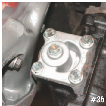
Photo #3a & 3b: The Delphi box includes new bolts to attach the box to the frame. With the box bolted to the frame, the clearance between the box and the exhaust is the same on the Delphi box and the original one. The Delphi box is taller than the original box at the firewall. If the stock mast jacket is going to be used, P/N 53-400 mast jacket conversion for column shift or 53-401 for floor shift (refer to CCI web site for a copy of the tech article) will need to be used.
