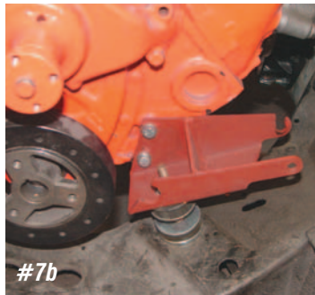
Photo #7a & 7b: Remove the stock left front motor mount and replace it with bracket P/N 53-27 . The new bracket is held to the engine block with the supplied grade-5 bolts and lock washers.
