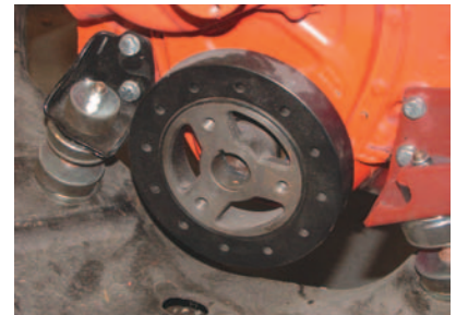
Photo #12: The bolt-on crankshaft pulley P/N 53-34 will drive the power steering pump. If the engine has the stock harmonic balancer with the riveted-on pulley, it will need to be updated with a pulley that accepts bolt-on pulleys. P/N 18-35 is a 6-1/8" diameter harmonic balancer that will accept bolt-on pulleys.
