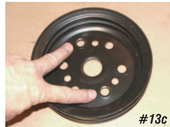
Photo #13a & 13b & 13c & 13d & 13e: The crankshaft pulley for the power steering pump P/N 53-34 is the third groove pulley for the crankshaft. This pulley is made to fit inside a single or double groove pulley. The double groove pulley P/N 51-03 has two collars that will key into the single groove pulley P/N 53-34 . With the pulleys keyed together, they can be bolted to the harmonic balancer.
