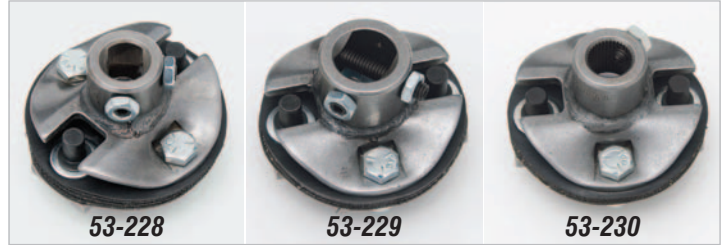
Photo #4: A flex coupler (rag joint) is used to connect the steering box to the steering column to improve road feel by reducing the transfer of bumps and vibration to the steering wheel. Three different couplers are available so the stock column or any aftermarket column can be used with the Delphi box. The bottom of each of the couplers is 17 millimeter female to connect to the steering box. The top of each coupler is where the difference is. Follow the chart below to determine the correct coupler to be used for your particular application.
