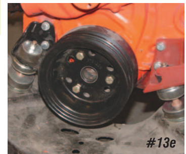
Photo #13a & 13b & 13c & 13d & 13e: The crankshaft pulley for the power steering pump P/N 53-34 is the third groove pulley for the crankshaft. This pulley is made to fit inside a single or double groove pulley. The double groove pulley P/N 51-03 has two collars that will key into the single groove pulley P/N 53-34 . With the pulleys keyed together, they can be bolted to the harmonic balancer.
