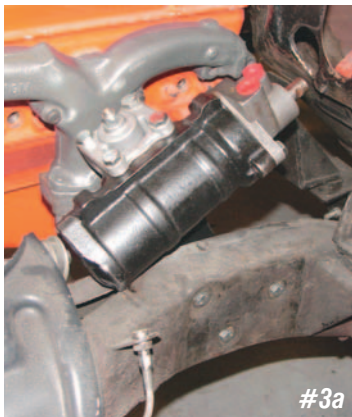
Photo #2a & 2b: The new Delphi power steering box has a one piece case and is bolted to the frame using the original three holes in the frame. The input shaft on the Delphi box is a male 17 millimeter double-D.
