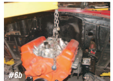
Photo #6a & 6b & 6c: The original front motor mounts attach to the front of the engine on each side of the harmonic balancer. The driver's side mount will be replaced with a combination left front motor mount and power steering pump mounting bracket. This bracket can also be used as the power steering pump bracket only if the engine is side mounted. Using an engine hoist or floor jack under the oil pan, slightly raise the engine to take the load off the front engine mounts.
