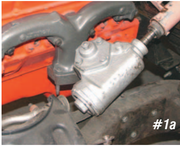
Photo #1a & 1b: The original steering box is bolted to the frame with three 3/8" carriage bolts and nuts. The stock mast jacket (steering column) protrudes through the firewall about 3-1/2". The steering shaft that connects the steering box to the steering wheel is part of the steering box and not removable.
