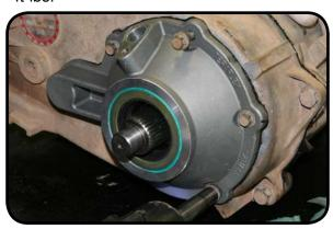
24. Install the new yoke. Use silicon on the splines of the yoke to create the seal. Use red thread locker on the yoke nut and torque to 100 ft-lbs.
