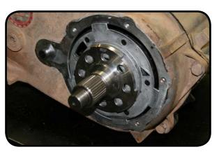
23. Install the new rear housing. Use silicon adhesive on the seal surface and torque to 20 ft-lbs.
