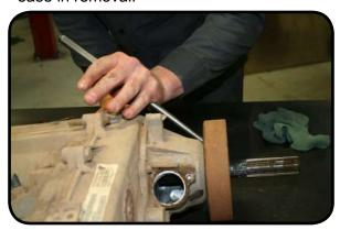
8. Remove the rear output shaft seal.
