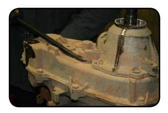
12. You will need to remove eight bolts to separate the transfer case. On seven bolts use a 15mm socket and the last bolt is a 10mm 12point that also needs to be removed. Now separate the two half using the pry slots that are machined into the case.
