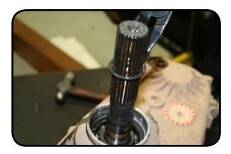
11. Remove the rear output housing using a 15mm socket and separate it from the transfer case.
