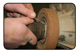
Remove the harmonic balancer (if equipped)
