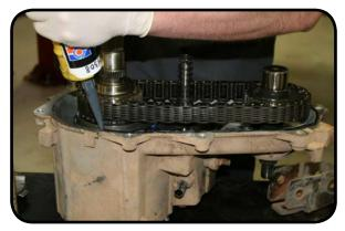
21. Install the rear half of the case. Make sure that the oil pick up and the magnet are installed in the case. Install the oil pump onto the shaft. Torque the bolts to 25 ft-lbs.
