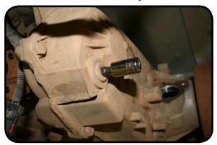
2. Remove the speedometer gear drive using a 13mm socket.
