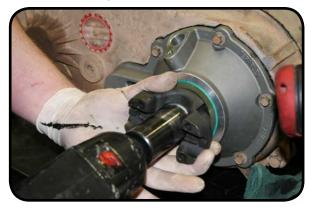
Install the new speed sensor into the tail housing using the supplied bolt and washer.
